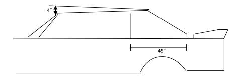
Sail panels and spoiler with supports to resemble this style. Sail panels cannot tie spoiler side supports.
